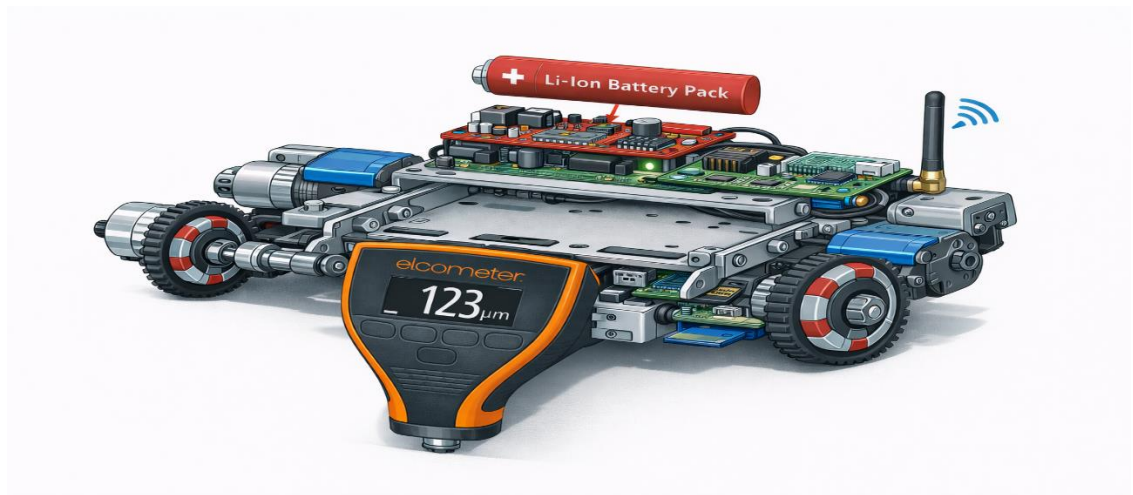
Figure 3: The assembled magnetic crawler device for DFT measurement.
